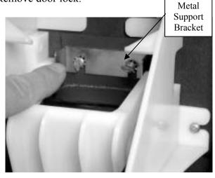
4 Loosen the two thumbscrews of the metal support bracket.
